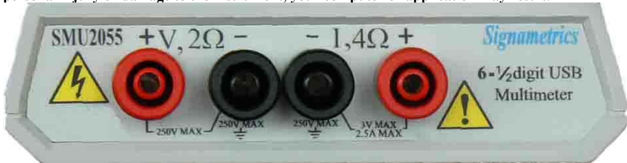
Figure 3-1. The DMM input connectors consist of four Banana jacks.
